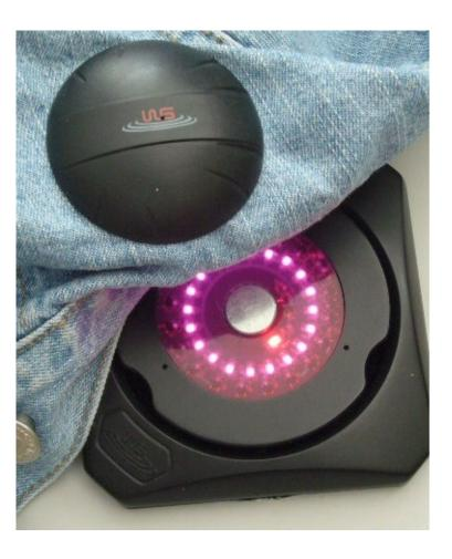
IR Pebble Tag is a four-alarm tag to protect high fashion products product's. Like in conventional tags a smooth groove less polished pin is stitched through the garment and thus the tag is positioned.
