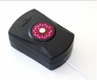
Opens Wave tags with IR code-protection and superlock magnetic lock
